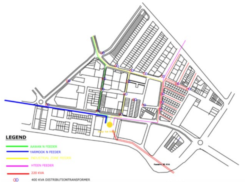
Figure 1. Planned Electrical Distribution Network
